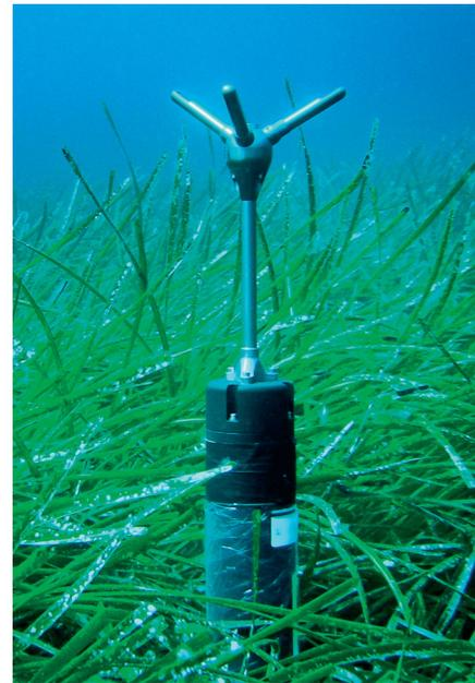
Fig. 2. Acoustic doppler velocimeter (ADV) deployed in the *Posidonia oceanica* seagrass meadow
