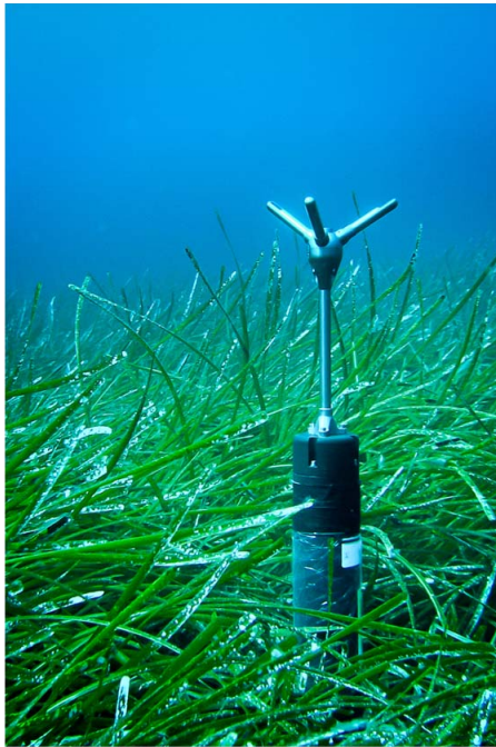
Figure 5.2: Acoustic doppler velocimeter (ADV) deployed in the Posidonia oceanica seagrass meadow.
