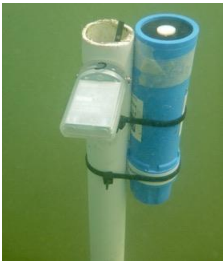
Figure 2.7 Light Meter. The picture shows a lux meter (Onset Hobo) and a PAR meter (Odyssey) mounted with cable ties on a PVC pipe at 2 m depth. Photo: P. Moksnes.
