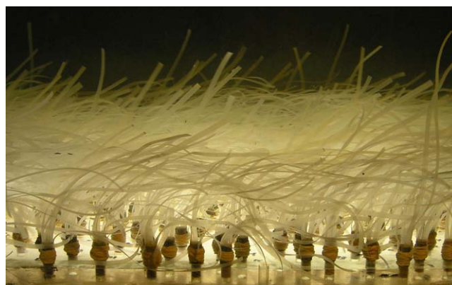
Figure 4. Photo of the model canopy with wave approaching from the left. The seagrass density is 1800 stems \text{m}^{-2} . The stem protrudes approximately 1 cm above the baseboards into the water. The mean measured diameter of the stems was d = 7.8 mm.
